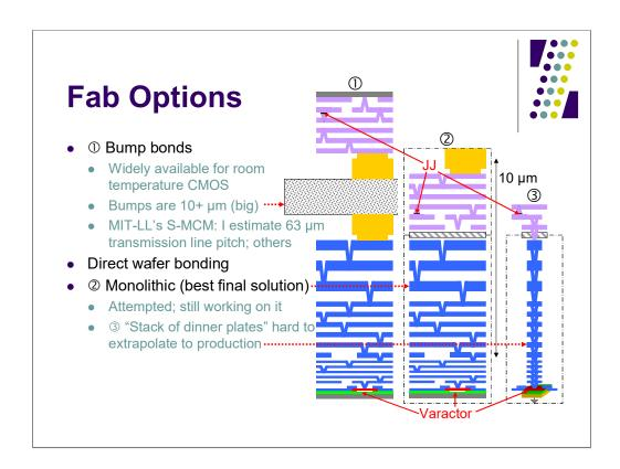
① illustrates bump connections. The blue stack is Google's open (Sky130) CMOS stack and purple is a MIT-LL superconducting stack. ① shows separate CMOS and a superconducting stack fabricated separately. The superconducting stack flipped over and the two are connected with bump bonds. This could work, but the bump bond is pretty big. MIT-LL has a superconducting multi chip module (S-MCM), which can move SFQ pulses through superconducting wires (but the actual bumps are normal metal).
