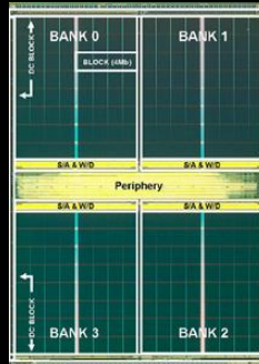
512Mb PRAM (Prototype) 0.1um 1.8V
