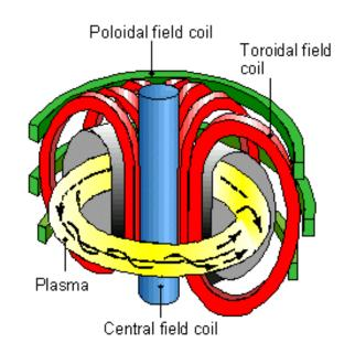
Charged particles have helical orbits in a magnetic field; they describe circular orbits perpendicular to the field and free-stream in the direction of the field.
