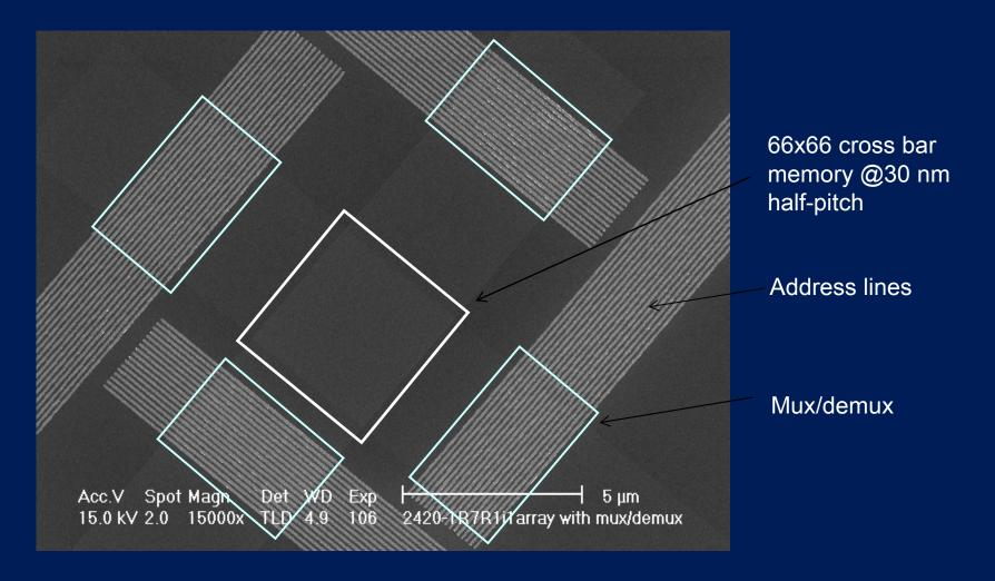
\*Mux/demux propramming done by E-beam burning
